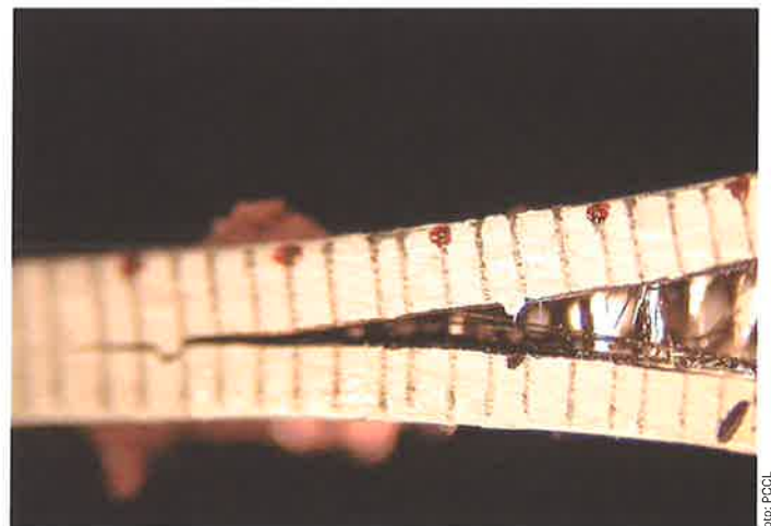
Kompetenzzentrum Polymer Engineering: Interlaminar crack propagation in a z-reinforced laminate
